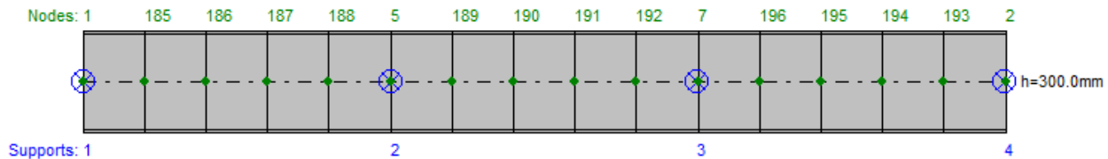
Figure 4: Defining lateral supports in AxisVM13
